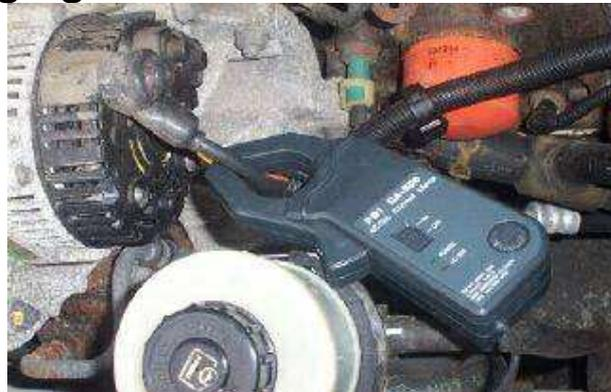
The clamp needs to be positioned around the wires on the back of the alternator. If this is not possible, then the clamp can be positioned at the battery positive cables. If possible, identify the wire that connects the alternator to the battery. With all the positive wires clamped at the battery, the clamp will read a balance between loads and the charging current.
