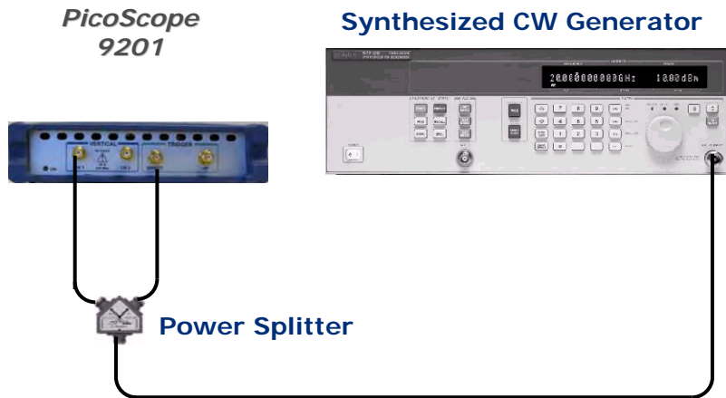
Equipment connections for Direct Trigger Test
