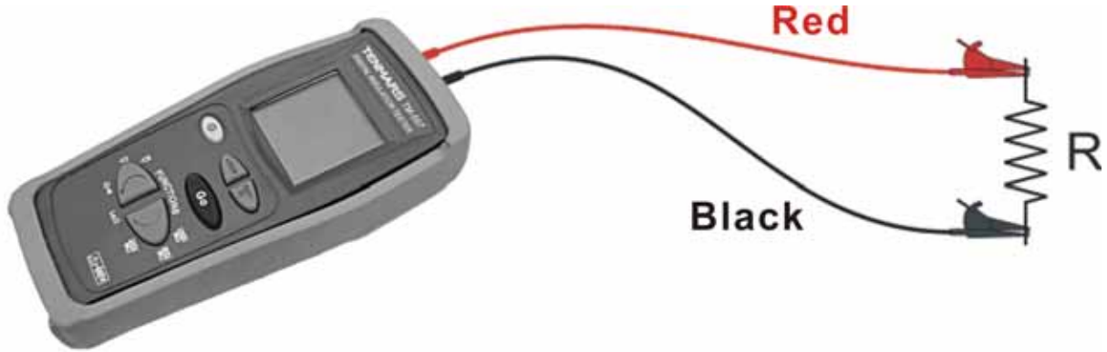
Fig. 4: Connection of the instrument's terminals during \Omega test
