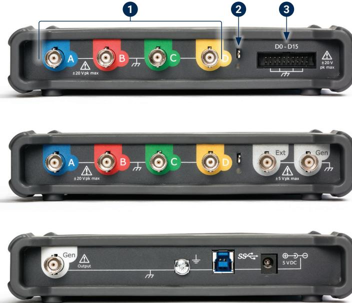
Note: PicoScope 5000D Series 4-channel models are shown here. Other models may have a different arrangement of connectors. Refer to your oscilloscope's data sheet for details.
